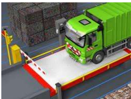
Figure 4: Weighbridges are key points to generate electronic waste transfer notes
