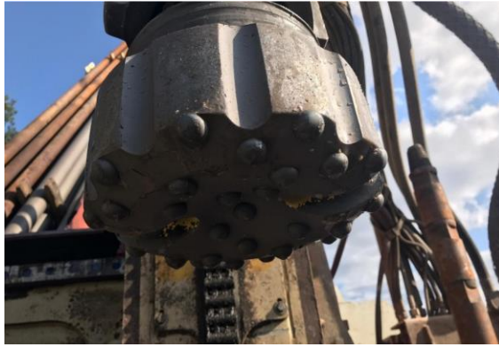
Fig. 31. Drill bit of the drilling machine for middle-deep geoenenergy wells. Photo. Vantaan Energia.
